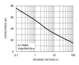
Fig.2 Typical Junction Capacitance
